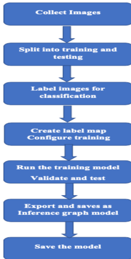
Fig 14 – Flowchart for Helmet Model
