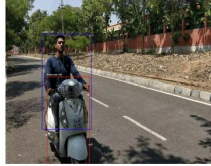
Fig. 2 (b): Frame with 'person' and 'motorcycle' classes detected (Case 2)
