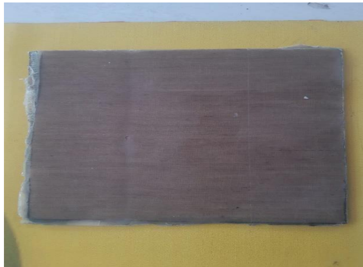
FIG.4.14 Composite Material Of (Ramie Fiber & Abaca Fiber)
