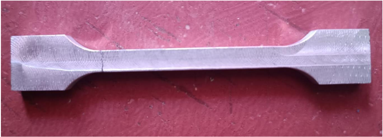
Fig:4.7: After grinding in according to ASTM Standard tensile specimen
