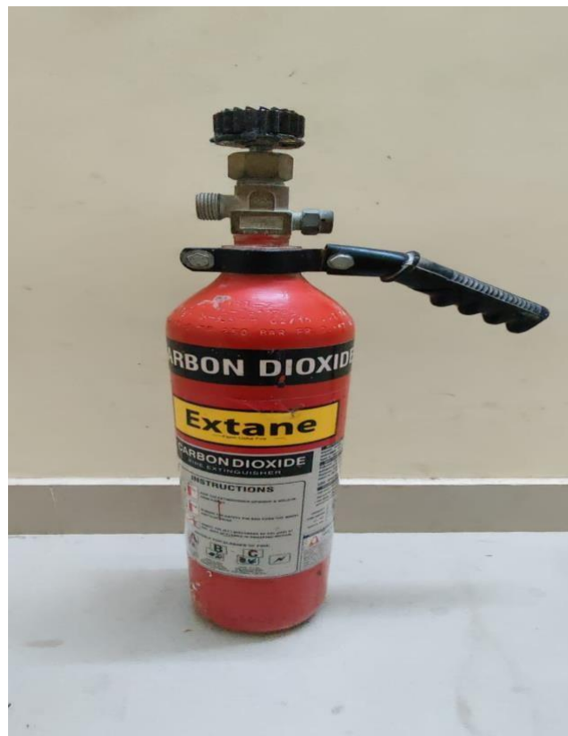
Fig :4.14 final customized cap mechanism of CO2 fire extinguisher
