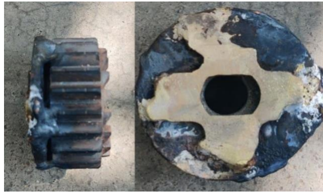
Fig 4.5: side and top view of grinded ring gear
