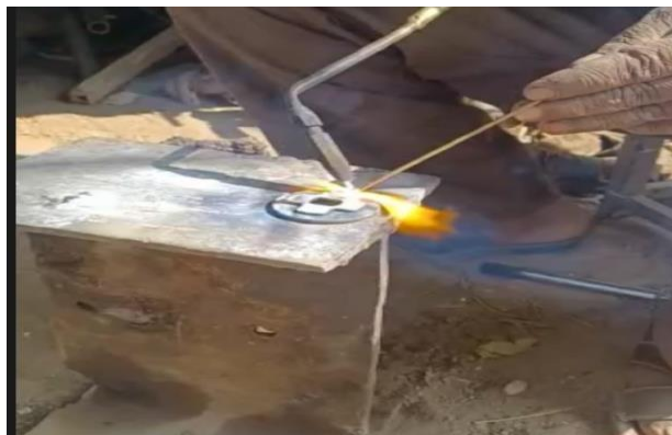
Fig :4.1 gas welding of ring gear
