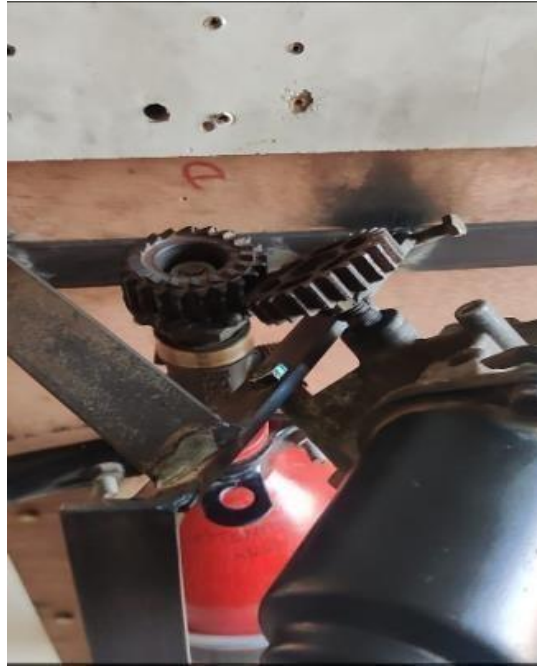
Fig 4.3: Gear assembly of wiper motor and CO2 fire extinguisher
