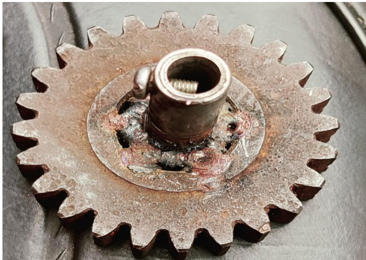
Fig: 4.2 welded gear for wiper motor
