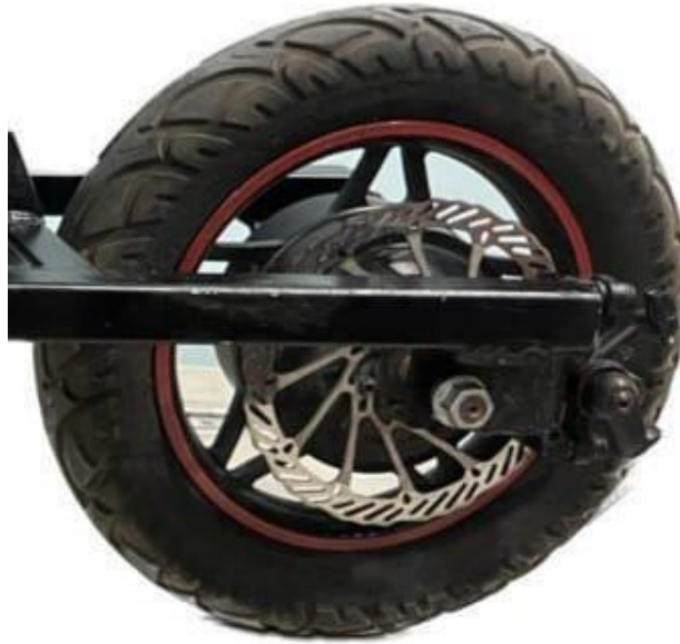
Fig 5.9 36v 250w BLDC hub motor
