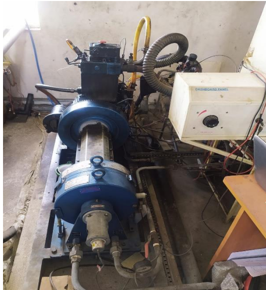
Fig. 1. 8. Kirloskar Engine TV 1 test setup
