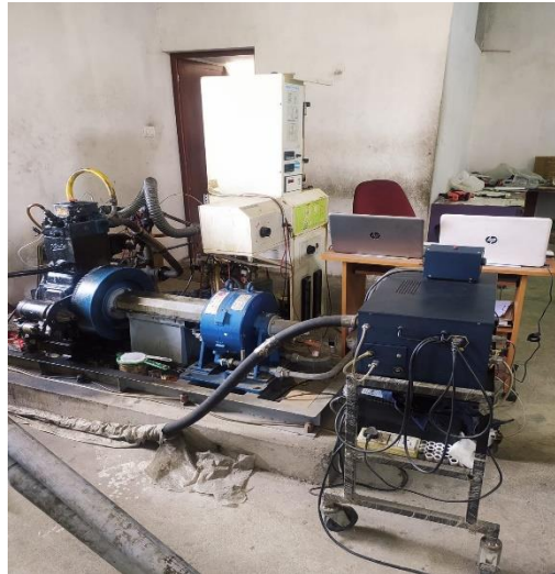
Fig. 4. 13. Engine testing in bio-oil with diesel blends
