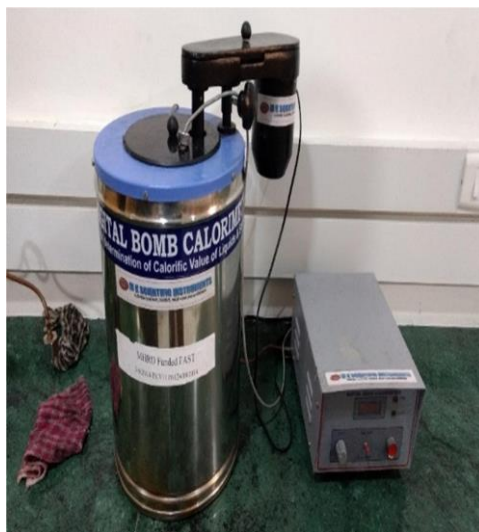
Fig. 4. 11. Calorific value measurement
