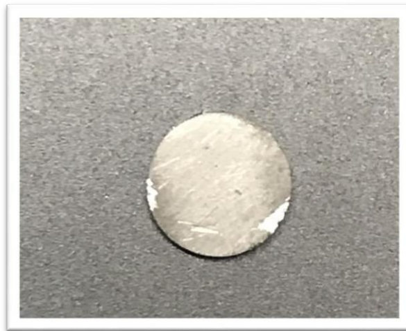
Fig:4.3 :sample size 2mm thickness 8mm diameter
