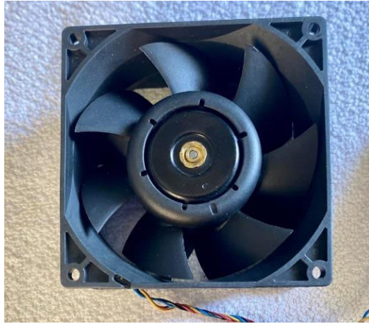
Fig. DC Brushless type motor with propeller blade.
