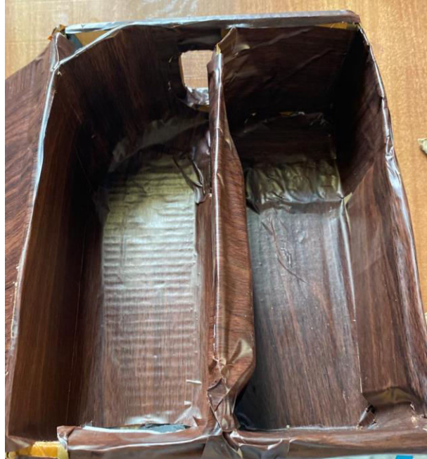
Fig. Casing with two chambers for vacuum and battery
