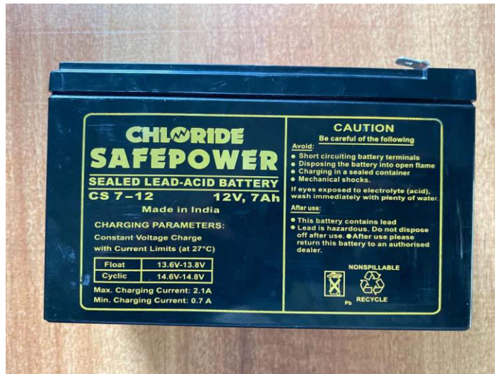
Fig. UPS Battery (12V)
