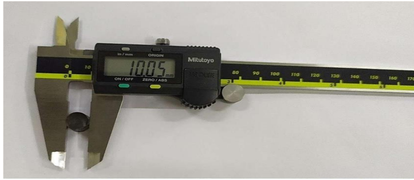
Figure: 6.1 Diameter of brake pad pin measured before heating
