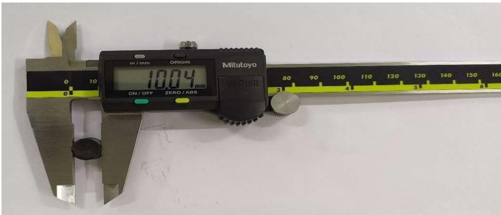
Figure: 6.5 Diameter of brake pad pin measured after water exposure
