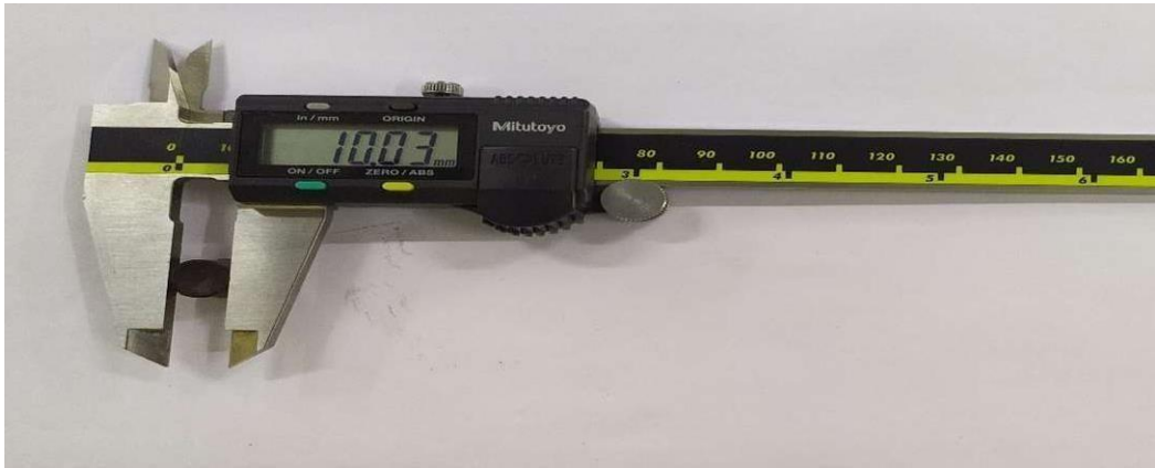
Figure: 6.4 Diameter of brake pad pin measured before water exposure
