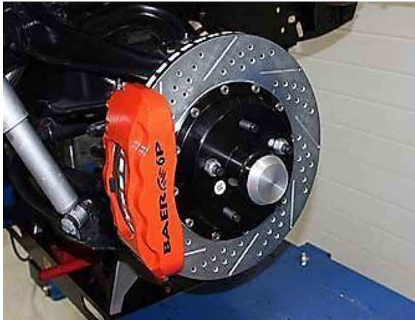
Figure: 1.2 A typical Disc Brake system with Brake pads
