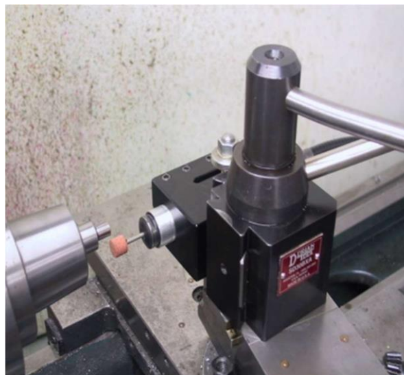
Figure: 5.8 Finishing process
