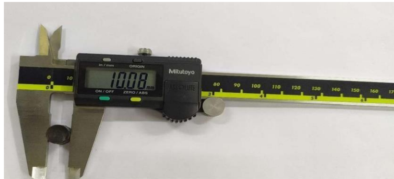
Figure: 6.2 Diameter of brake pad pin measured after heating
