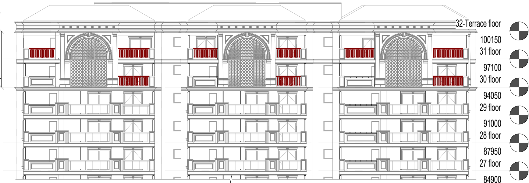
1 BALUSTER RAILING - EAST ELEVATION (TIER 4) SCALE 1 : 250
