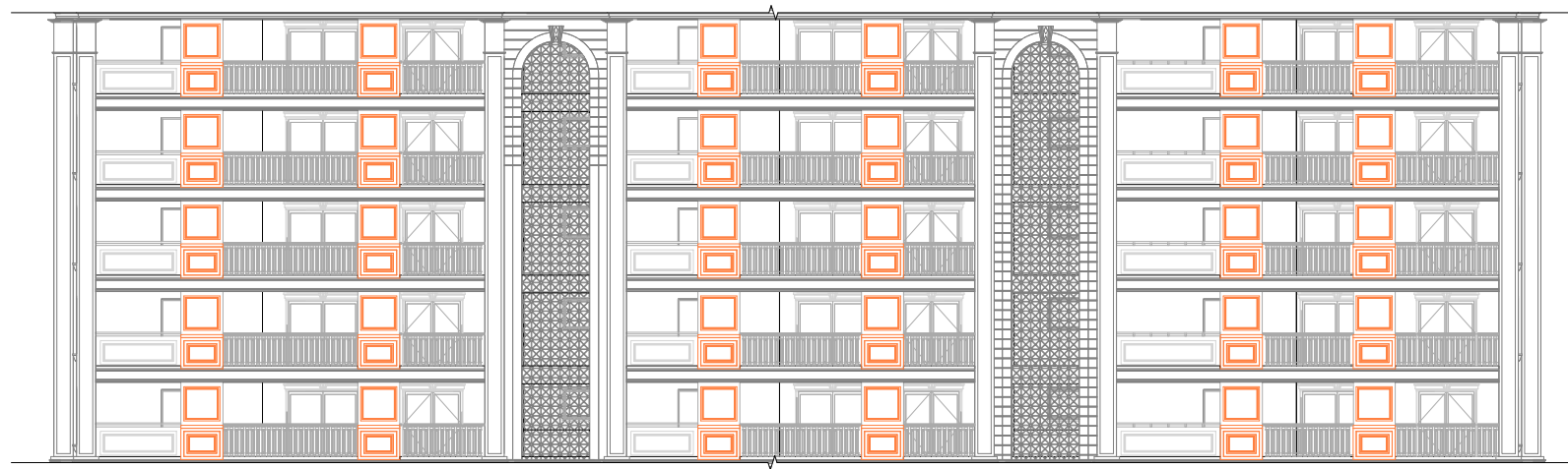
1 BALCONY ELEMENT - EAST ELEVATION (TIER 2) SCALE 1 : 250
