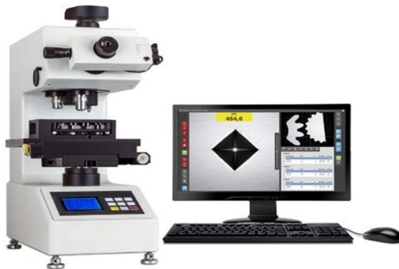
Fig 2.5 Experimental setup of Vickers hardness test
