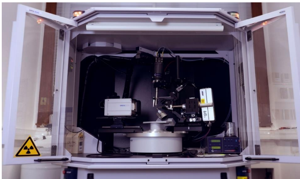
Fig .2.2 Instrumental setup of BRUKER KAPPA APEX 2
