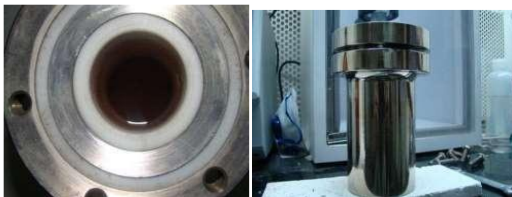
FIG. 4.2 Autoclave for solvothermal synthesis.
