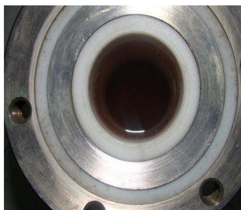
FIG:4.2 This is called Teflon which is used to pour the solution and kept in Autoclave for solvothermal synthesis.
