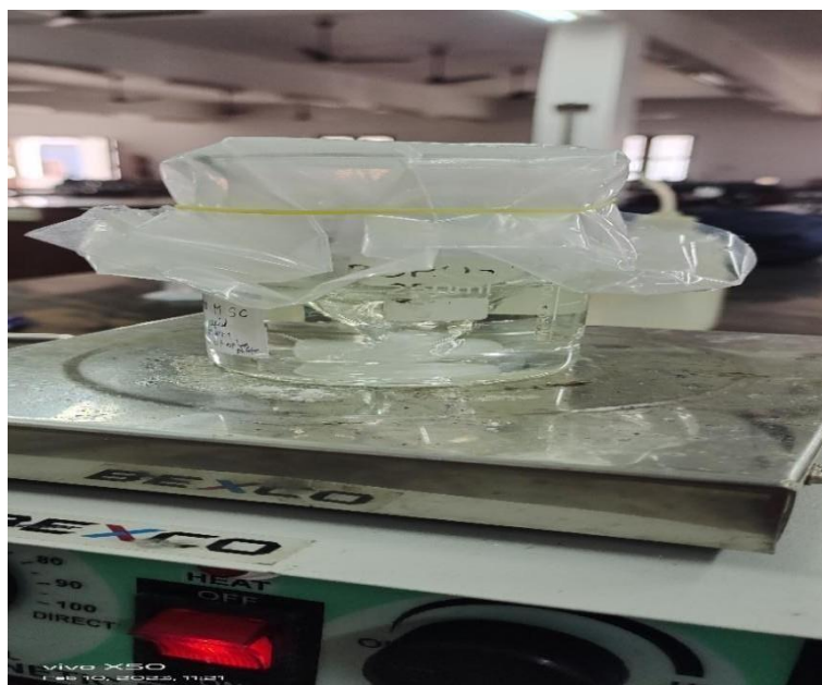
Fig 5 synthesis of CNP using magnetic stirrer
