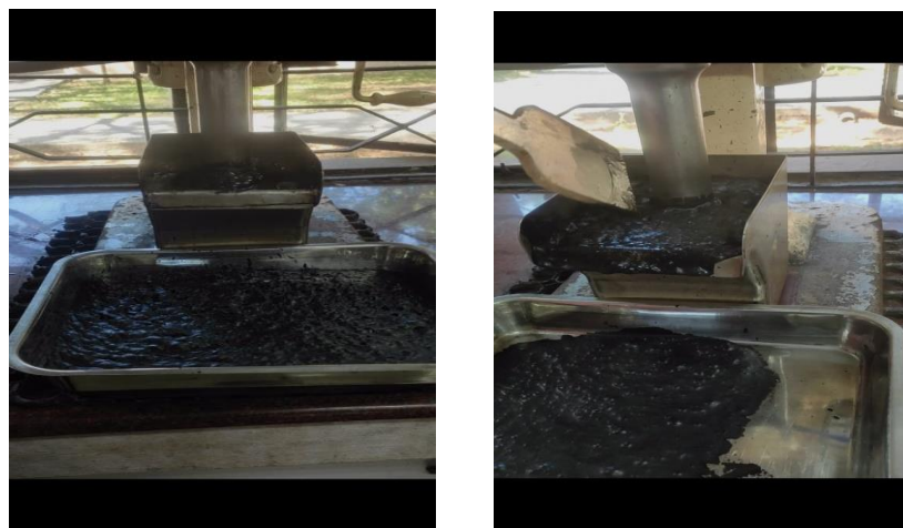
Fig.4.8. Froth obtained from flotation of non-coking coal
