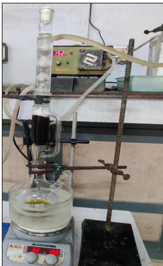
Fig.4.3. Soxhlet extraction setup
