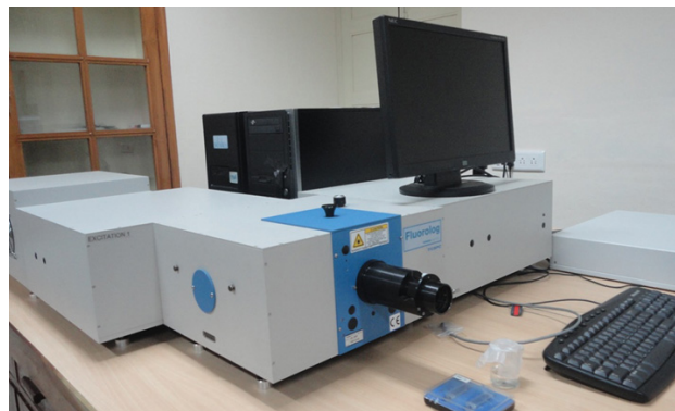
Fig.4.2.2.3. Time-Related Single Photon Counting (TCSPC) [Fluorolog – 3] (Department of Medical Physics, Anna University)
