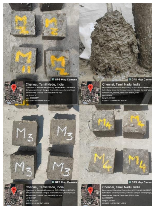
Fig. 3.5: Casting of cubes and workability
