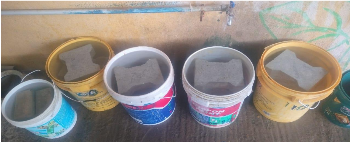
FIG. 3.6 CURING OF I SHAPED PAVER BLOCKS
