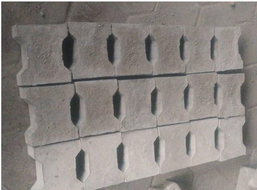
FIG. 3.5 DEMOULDED I SHAPED PAVER BLOCKS
