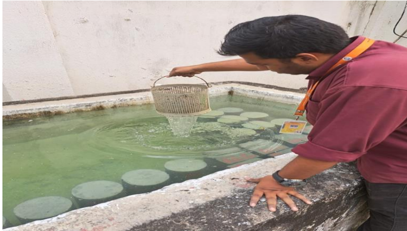
Fig 4.4 immersing coarse aggregate into the water
