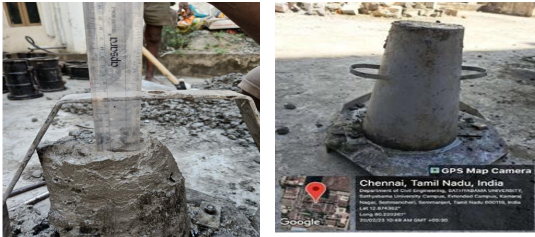
Fig 4.9 Slump cone Test
