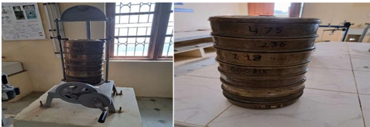
Fig 4.2 Fine Aggregate sample within the sieve & appropriate size of sieve
