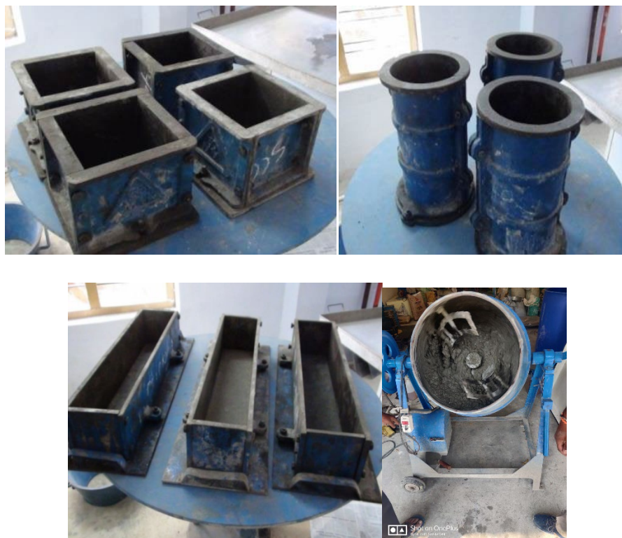
Fig 4.3 Cube, cylinder and beam mould with oil applied and casting process
