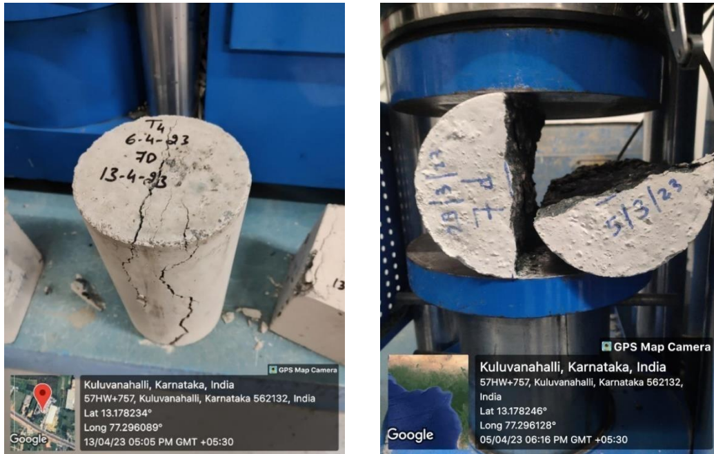
Fig 4.7 Cylinder specimen for split tensile.
