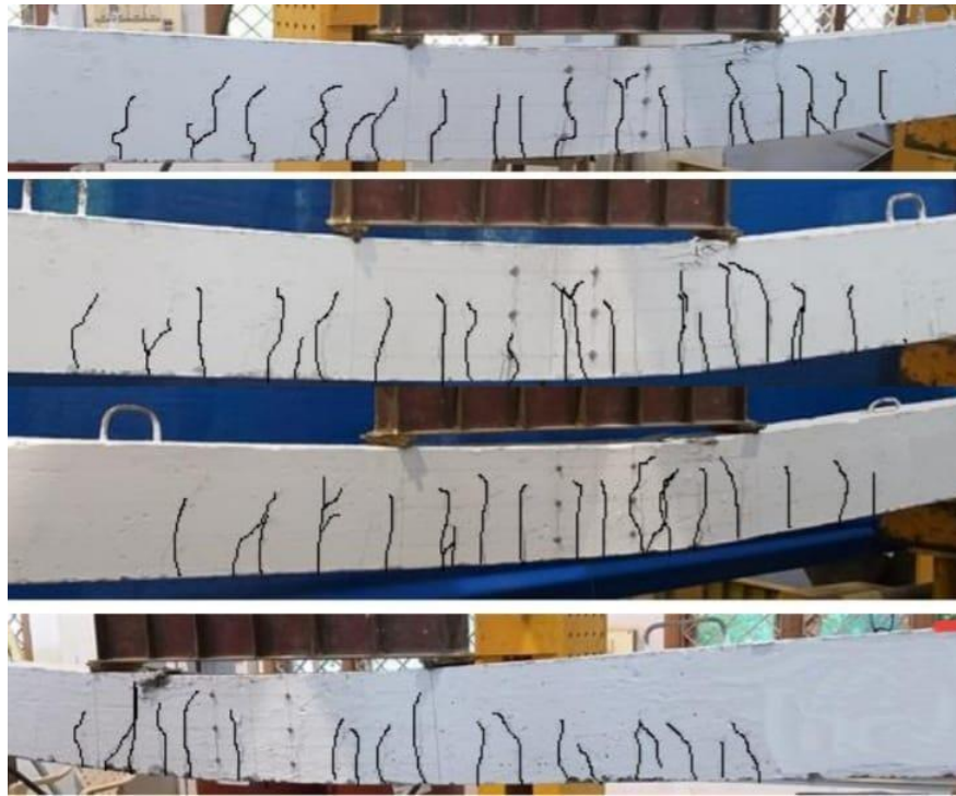
Fig 4.8 RCC BEAMS IN TWO-POINT LOADING (a)GPB (b) GPC TYPE 1 (c) GPB TYPE 2 (d) GPC TYPE 3
