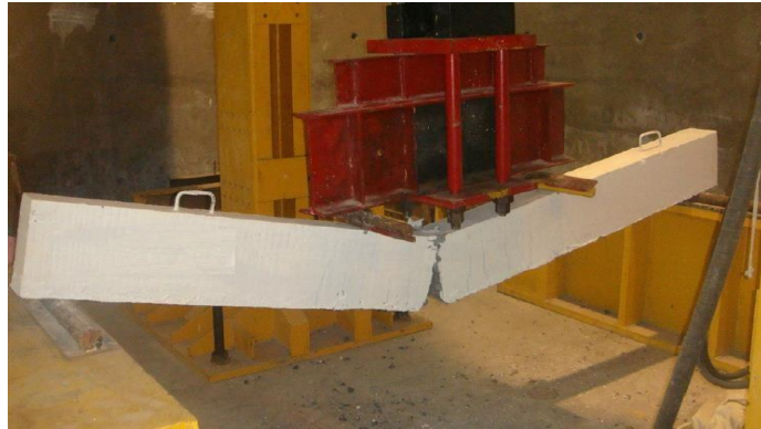
Fig 4.14 Loading Frame Setup with Conventional Beam
