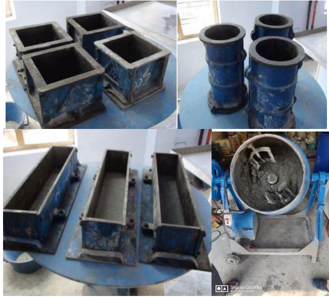
Fig 4.2 Cube, cylinder and beam mould with oil applied and casting process
