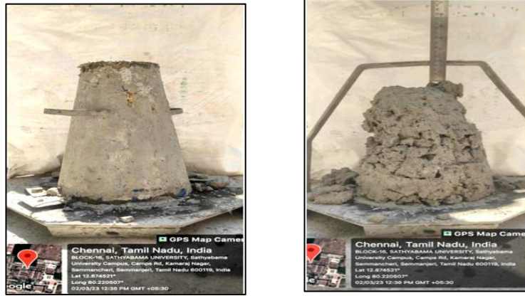
Fig 4.11 Slump cone test
