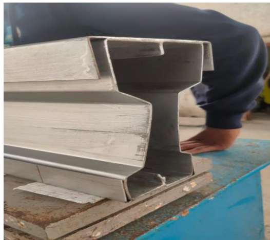
Fig 4.12: MSTT After Applying Load
