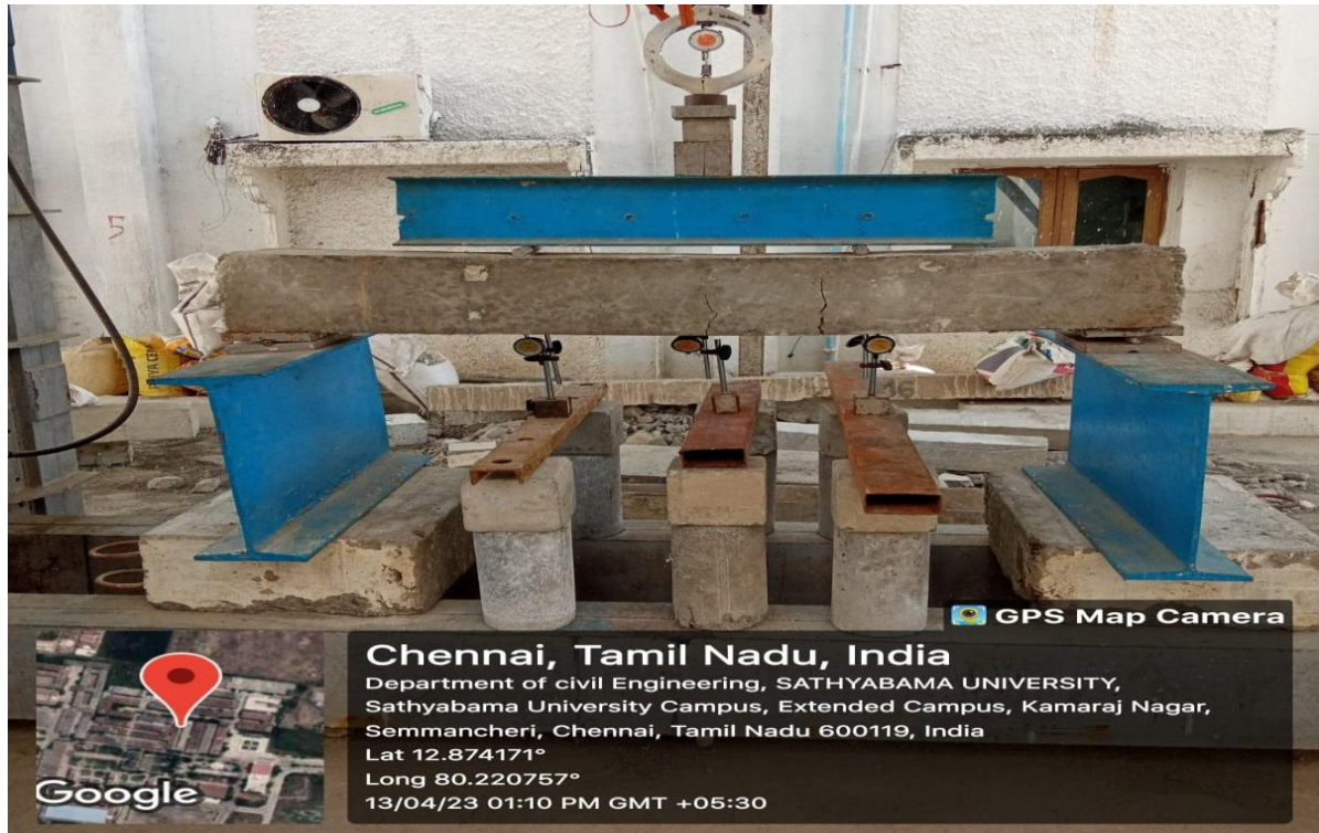
Fig 5.7: Flexural test for beam specimen
