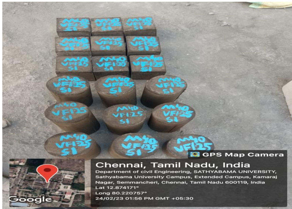
Fig 5.4: Casted Cube and cylinder specimens
