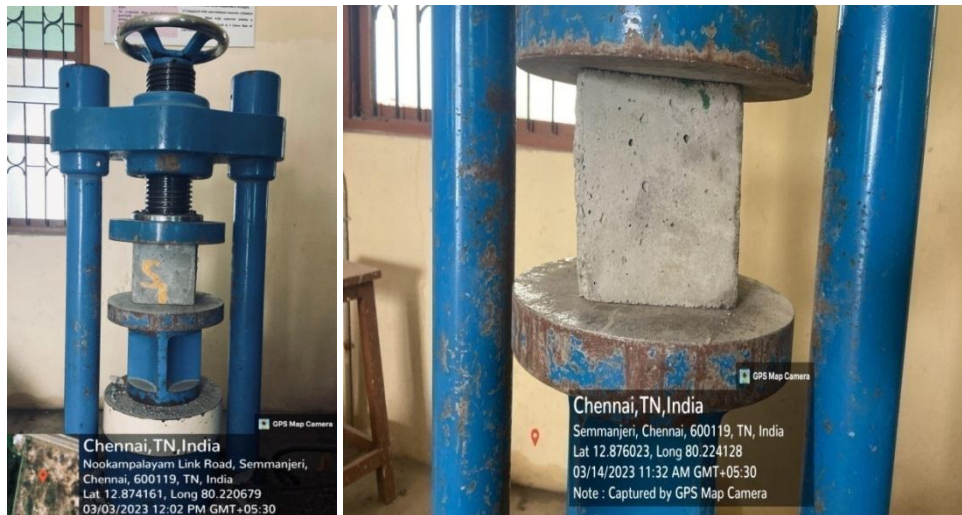
Fig.5.5 compression testing on cube specimen
