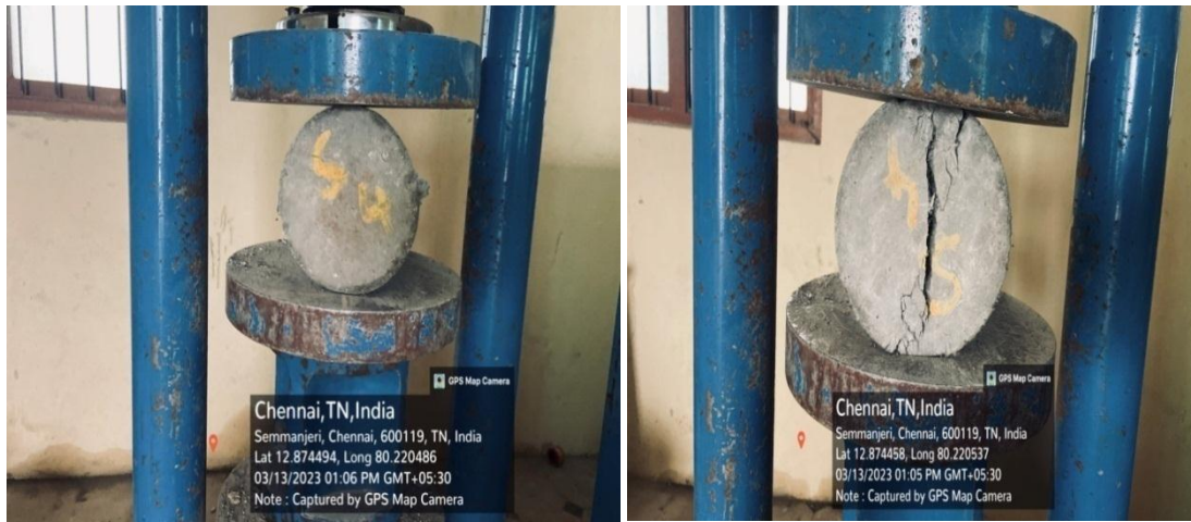
Fig.5.6 splitting tensile strength test on cylindrical specimen
