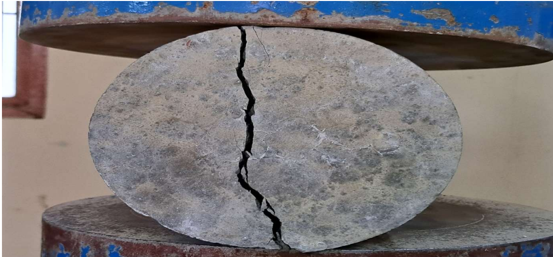
Fig 3.13 Cylinder Specimen in Split Tensile Strength Test
