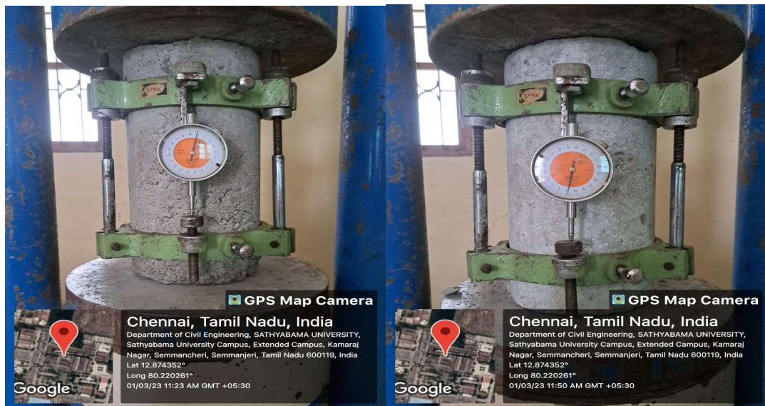
Fig 3.14 Young's Modulus Test on Concrete
