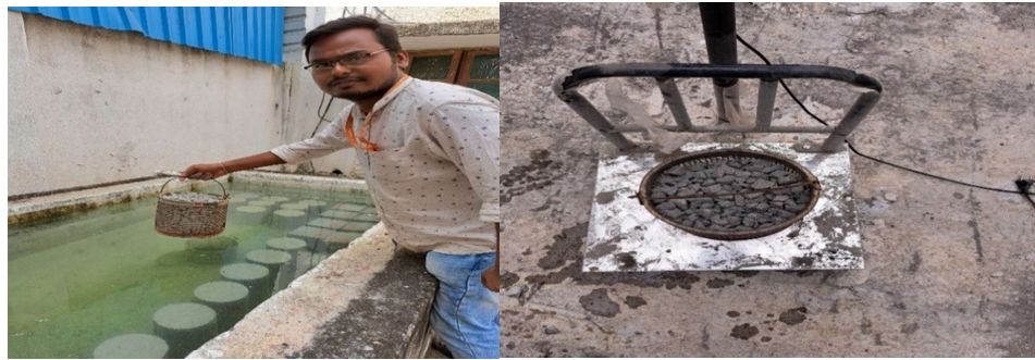
Fig 3.7 Specific Gravity and Water Absorption Test
