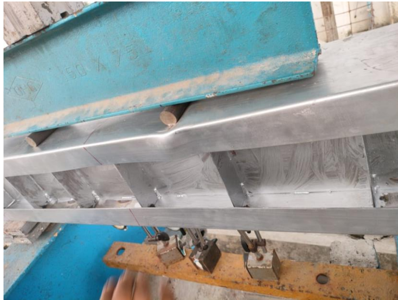
Fig 3.9: I Section beam after applying the load
