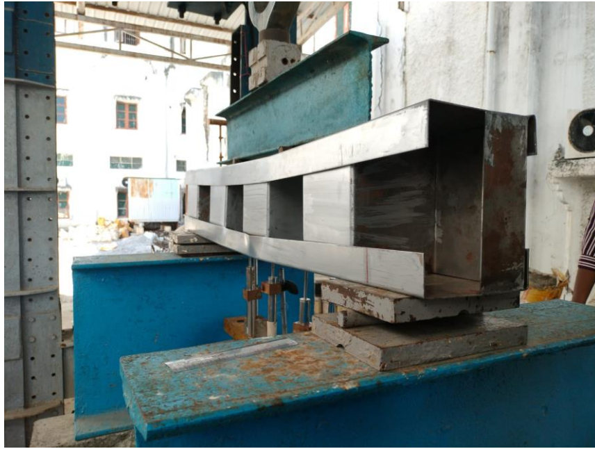
Fig 3.11: rectangular beam after applying the load
