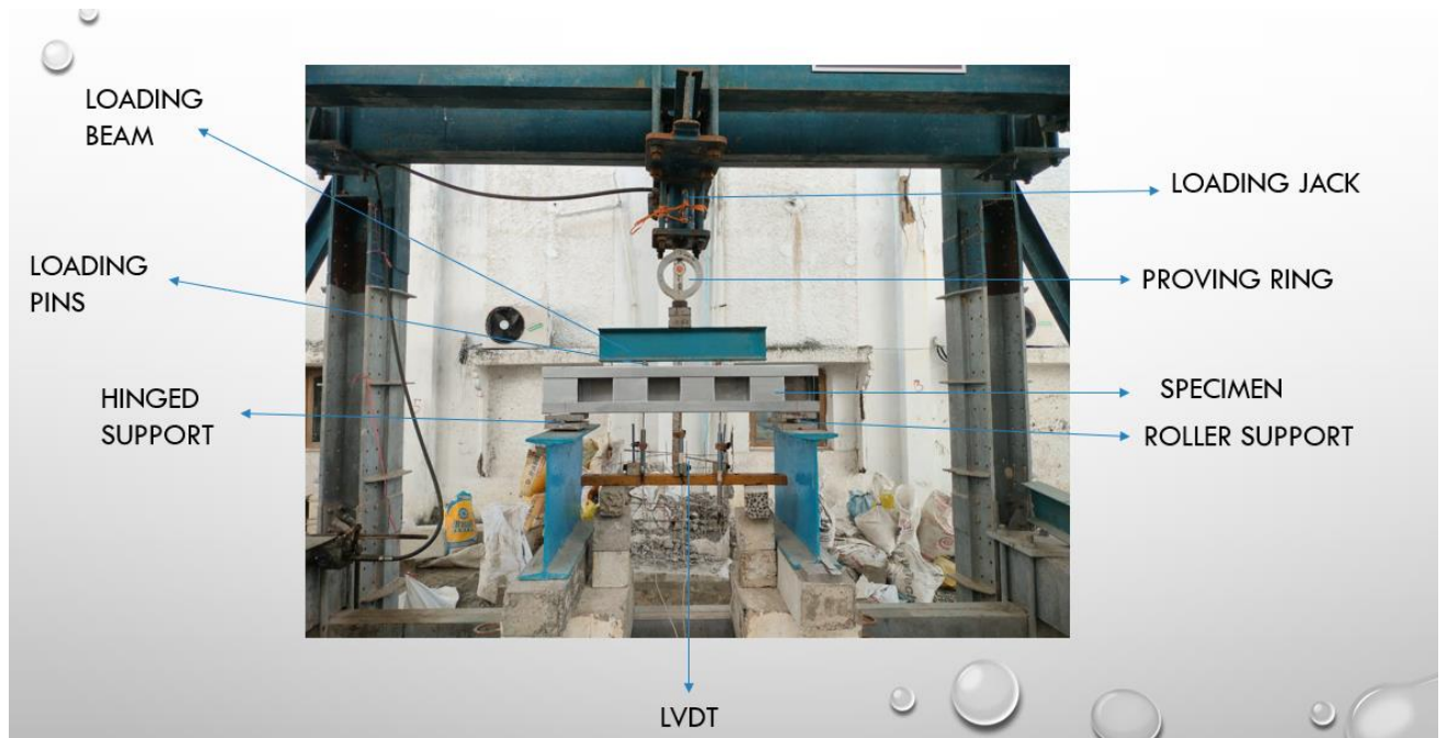
Fig 3.8 Loading frame setup for testing
