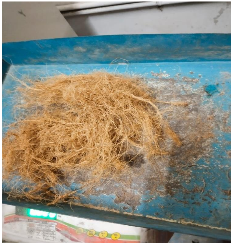
Figure 4.10 Coconut fiber separating process
