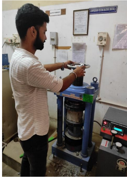
Figure 6.2 concrete block placed
