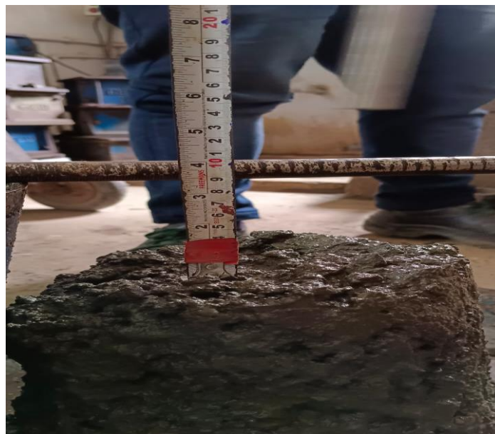
Figure 5.1 Slump cone test
