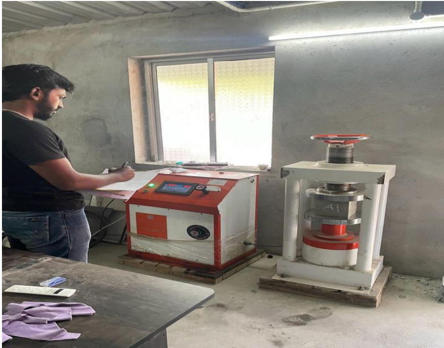
Figure 5.1: Compression test of concrete cube
