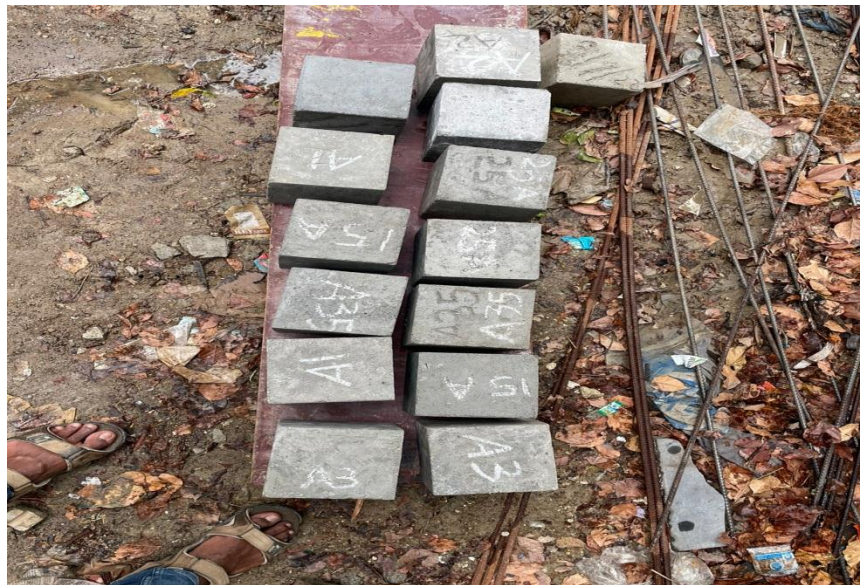
Figure 4.14: Removal of mould
