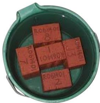
Fig 5.5 Water absorption test apparatus
