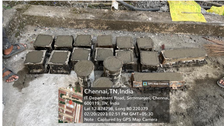
Figure 4.6 casting of concrete specimens
