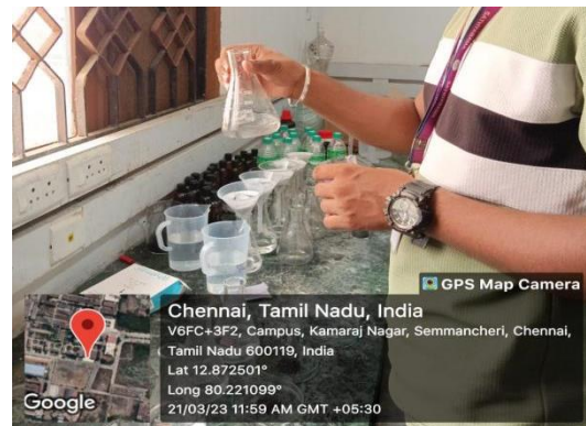
Figure 4.7 Adsorbents were mixed with the zinc ion solutions and kept for the adsorption process .
