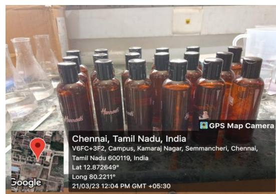
Figure 4.8 After the adsorption process sample was filtered and stored in the containers
