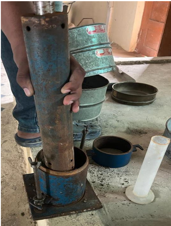
Fig:3.7: Compacting soil by giving blows
