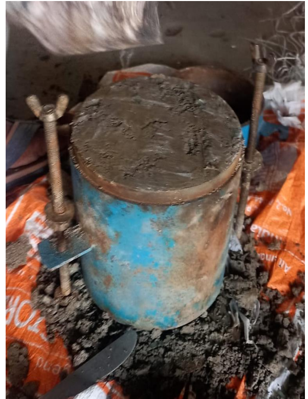
Fig:3.8: Soil after compaction
