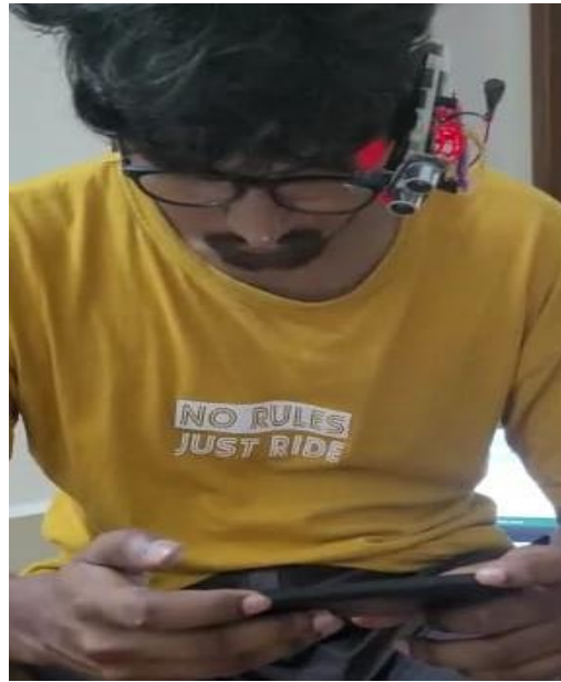
Fig: 5.2: The MPU 6050 gyroscope sensor detect the neck posture
