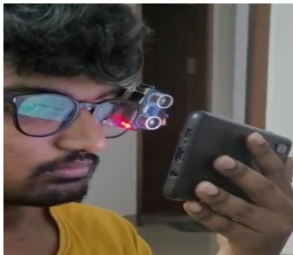
Fig: 5.5: The ultrasonic sensor sense distance between screen and user.
