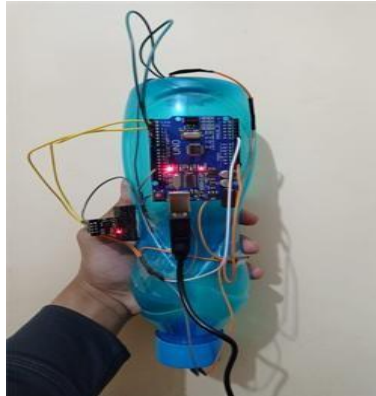
Fig 1.1 IV monitoring using ultrasonic sensor
