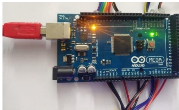
Fig. 4.20: Connection of USB cable to Arduino
