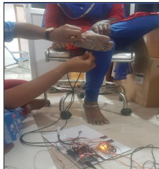
Fig 5.3 Measurement of Plantar Temperature using DS18B20
