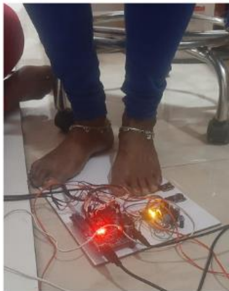
Fig 5.4 Measurement of Plantar Pressure using force-sensitive resistors
