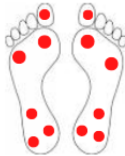
Fig 5.2 Representation of Sensor Locations for Data Acquisition
