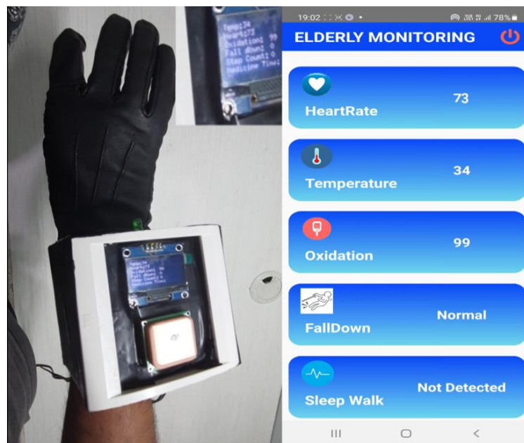
Fig .5.12: When the finger is placed on the sensor the oxidation and the heart rate are detected
