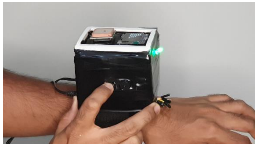
Fig .5.4: When the push button is pressed the LED starts glowing
