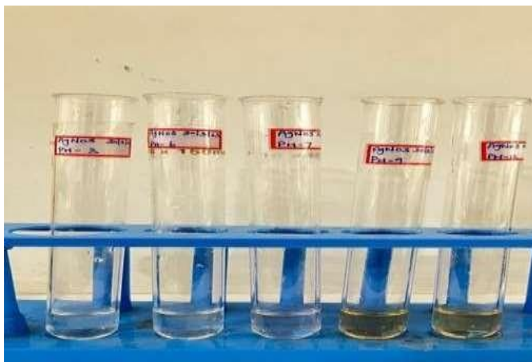
FIG 5.7: SYNTHESIS OF Ag NPs BASED ON DIFFERENT pH.
