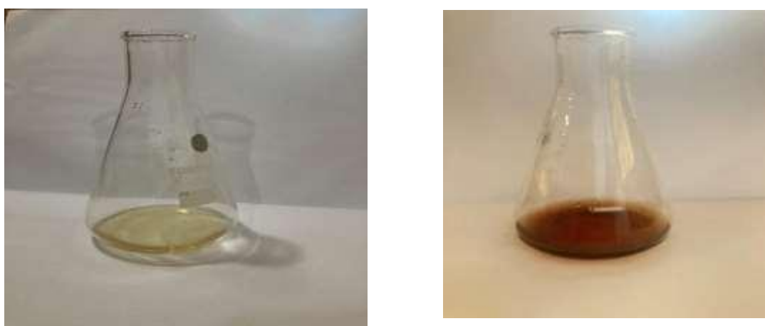
FIG 5.3: BULK SYNTHESIS OF Ag NPs WITH 0.05 MOLARITY, FORMATION OF Ag NPs BY COLOUR CHANGE.
