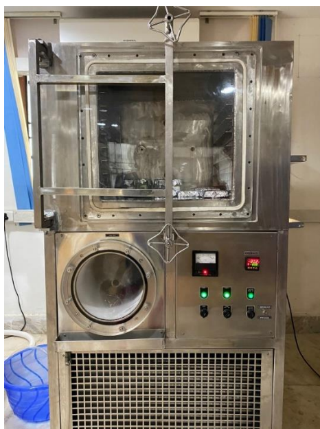
Fig. 5 Freeze- dryer set up for lyophilization of extracted protein samples for further protein analysis such as FTIR/ATR and Raman
