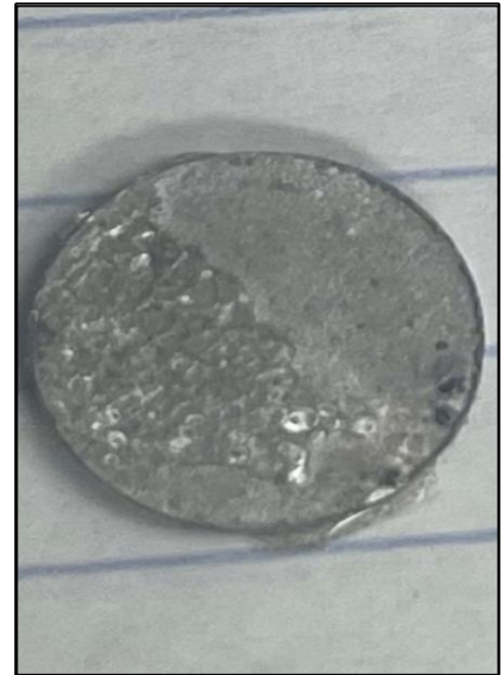
Figure 5.7.4 .1wt % fabricated mg implant with 10% polymer (sample B)
