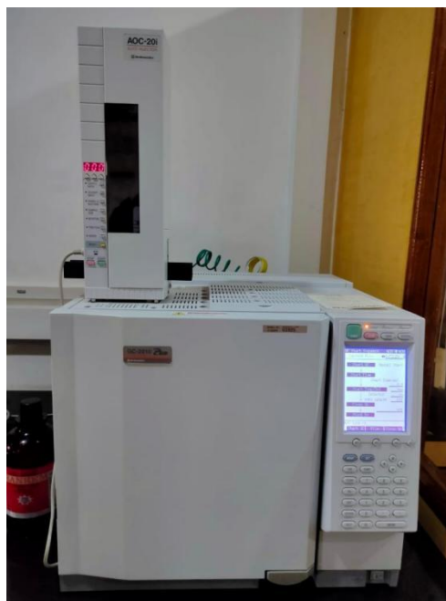
Fig 4.7: Gas Chromatography with Flame Ionization Detection (GC-FID). GC 2010 Plus.
