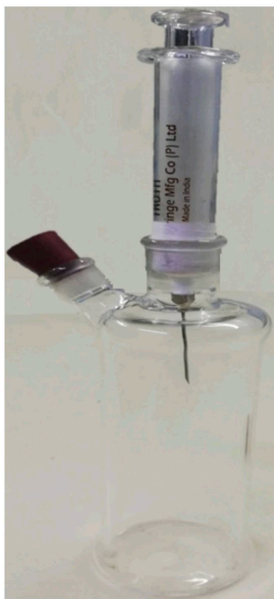
Fig: 4.4.1 Borosilicate Glass Photo reactor
