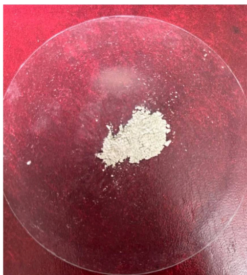
Fig 4.2.2.2 g-C 3 N 4 loaded with Pt
