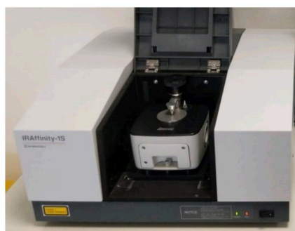
Fig 4.3.2 FTIR (Fourier Transform Infrared Spectroscopy)
