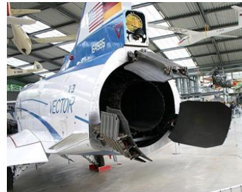
Fig 3.4 Examples of thrust vectoring that used the exhaust flow deflection technique.
