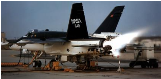
Fig 3.4 Examples of thrust vectoring that used the exhaust flow deflection technique.
