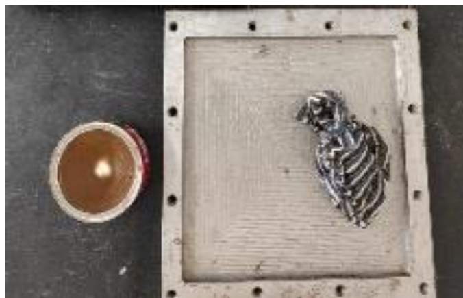
Fig.4.10: Wax applied on mould
