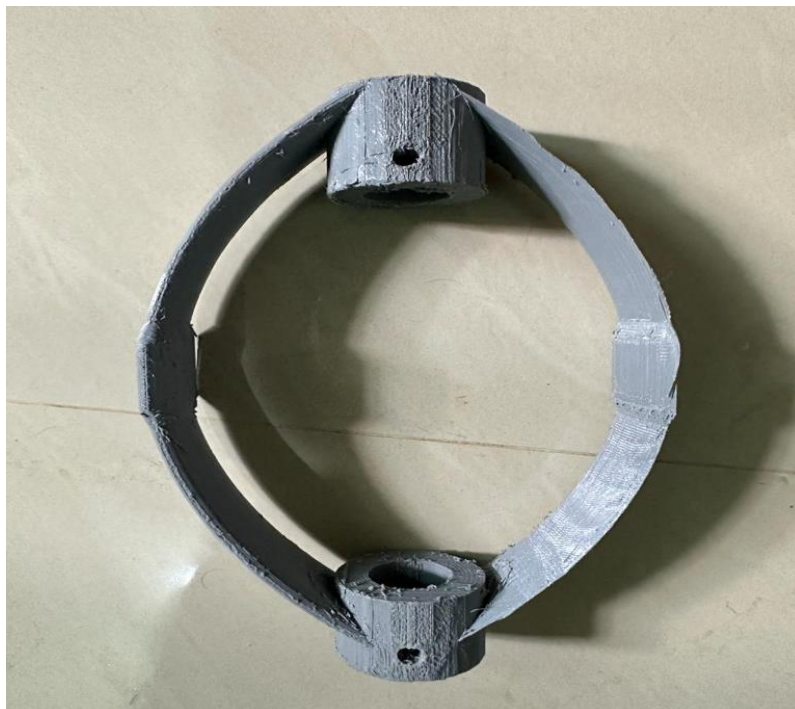
Fig: 4.12 : Fabricated Turbine
