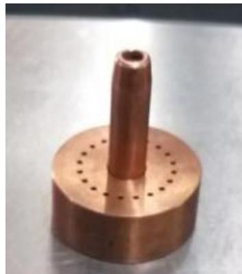
FIG 4.19 Assembly of Cathode.
