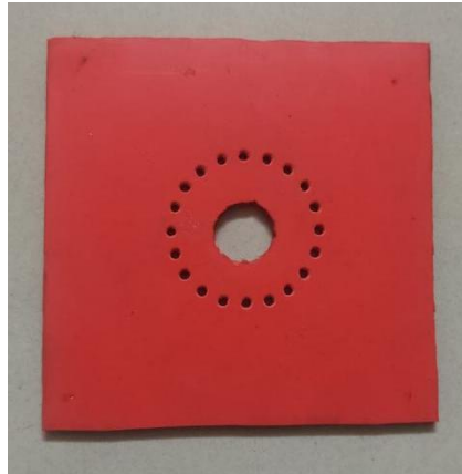
FIG 4.20 Insulator for Back of Cathode.
