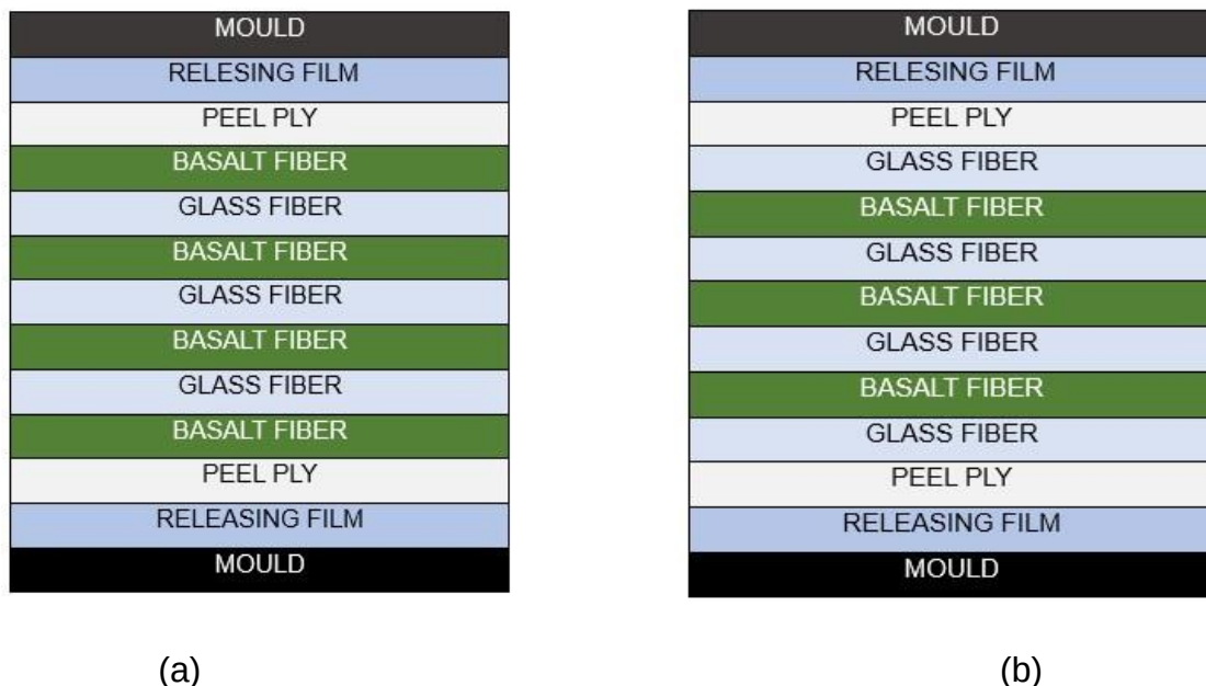
Fig.4.12: (a) Schematic diagram of Basalt –GFRP composite is prepared by replacing intermediate layers (b) Schematic diagram of GFRP-Basalt the composite is prepared by replacing intermediate layers.
