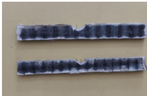
Fig.4.20: Glass/Basalt and Basalt/Glass Samples for impact test
